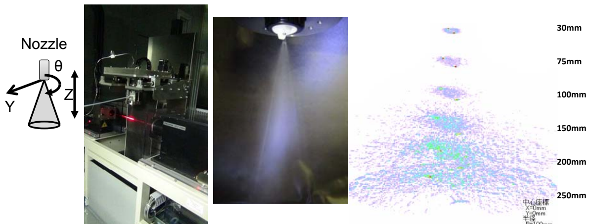
Fig. 3 3D spray structure and droplet size analyzer by laser CT technology
